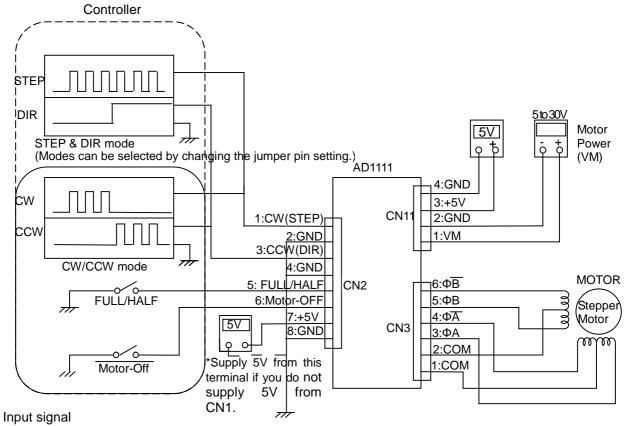
CW and CCW Driving pulses are input in these terminals. When pulses are input to CW terminal, the axis rotates in a clockwise direction. When pulses are input to CCW terminal, the axis rotates in a counterclockwise direction. The motor operates at the rising edge of pulse signals. Note 1.
