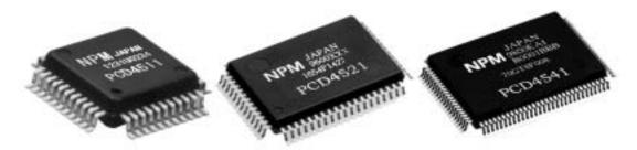
The PCD4511/4521/4541 are excitation control LSIs designed for 2-phase stepper motors. With just one of these LSIs and a stepper motor driver IC (e.g. NP-7026), you can easily construct a stepper motor control system.
